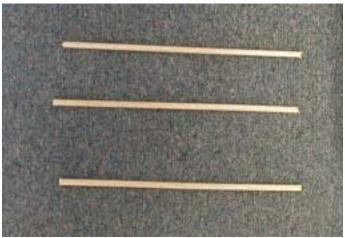
Cut 1/4" in diameter dowels to lengths of about 8 to 9" long.
